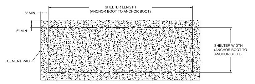
RECOMMENDATION: BRASCO RECOMMENDS A 6 INCH THICK 3000 PSI CONCRETE PAD. THE CONCRETE PAD SHOULD ALLOT A MINIMUM OF 6 INCHES AROUND THE SHELTER PERIMETER TO PREVENT CONCRETE BREAKAGE WHEN ANCHORING SHELTER TO PAD. CONCRETE MAY OR MAY NOT REQUIRE ADDITIONAL REINFORCEMENT. IF CONCRETE CALCULATIONS ARE REQUIRED FOR INSTALLATION OR PERMITTING PURPOSES, PLEASE CONTACT YOUR BRASCO ACCOUNT MANAGER FOR A QUOTE.
